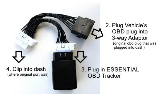
It is important to cable-tie or tape up the excess wires under the dash and to firmly secure the GPS to the
